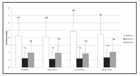
Method 1: 2 caregivers using old method of repositioning 246% greater exertion than SPS Method 2: 2 caregivers with SPS Method 3: 1 caregiver with SPS 52% greater exertion than method 2
